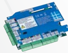
I-Net™ Supervised Door Controller
