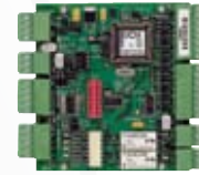
I-Net™ Reader Expansion Board
