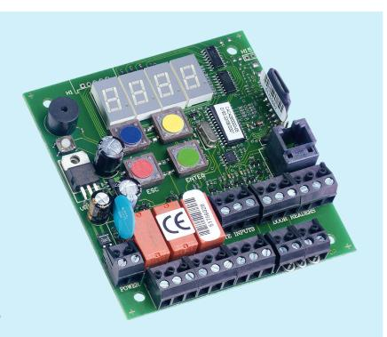
The Solo 2 from Controlsoft is a standalone Access Control Unit, providing cost effective access control for two door applications using Wiegand readers. Up to four readers can be connected giving you IN/OUT readers for two separate doors.
