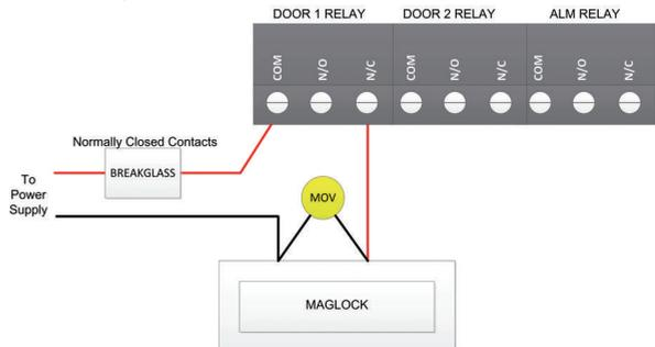
**ALWAYS FIT A MOV SUPPLIED WITH THE SOLO 2 ACROSS THE MAGLOCK TO AVOID BACK-EMF DAMAGING THE ACU**
