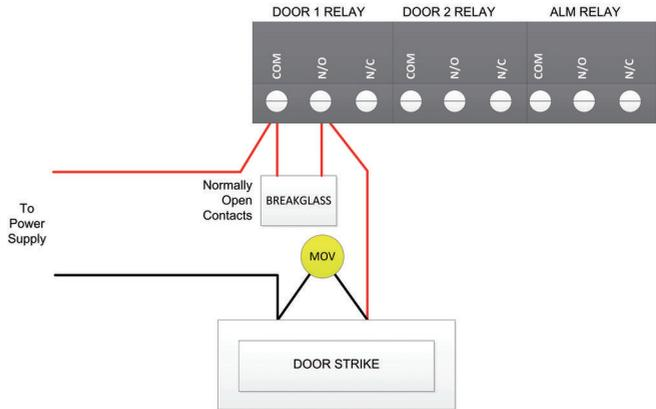
**ALWAYS FIT A MOV SUPPLIED WITH THE SOLO 2 ACROSS THE DOOR STRIKE TO AVOID BACK-EMF DAMAGING THE ACU**
