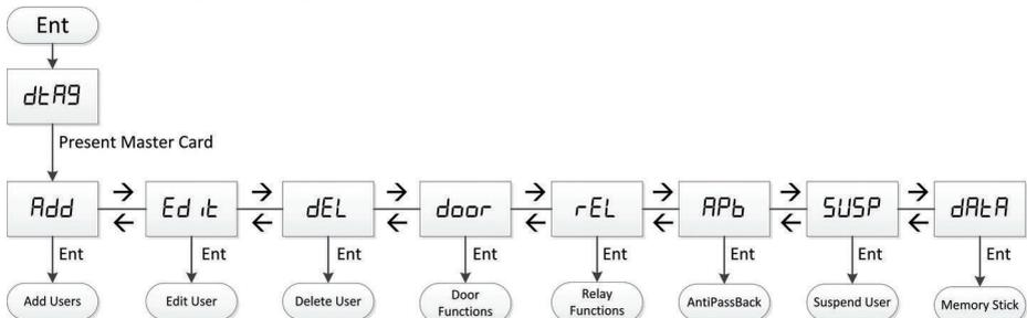
To enter programming mode, first press the ENTER button, and the display will show DTAG. Present the Master Card to the reader and the display will change to ADD. Press ---> to display EDIT, or ---> again to display DEL etc. When the display shows the desired function, press the ENTER button.
