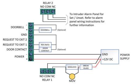
**NOTE**: A MOV **MUST** be fitted across any inductive load connected to the KP-800
