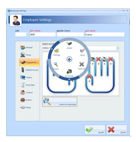
Place the selected finger on the enrolment reader 3 times, following the on-screen instructions where necessary.
